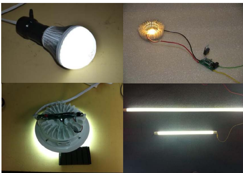
Figure 2: Various lights using MIK36XX driver
